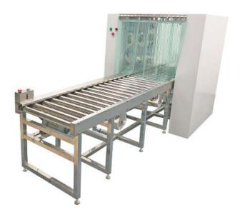
Air shower pass box between the clean area and the non-clean area, so as to reduce the number of times the clean room is opened and pollute the clean area. Reduce to a minimum.
